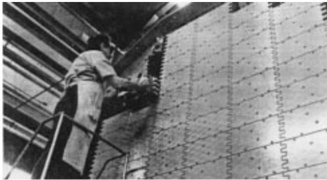
Fig. 11. AN/SPY-1 S-band passive array. The 32-element array modules are evident in the aperture face.
