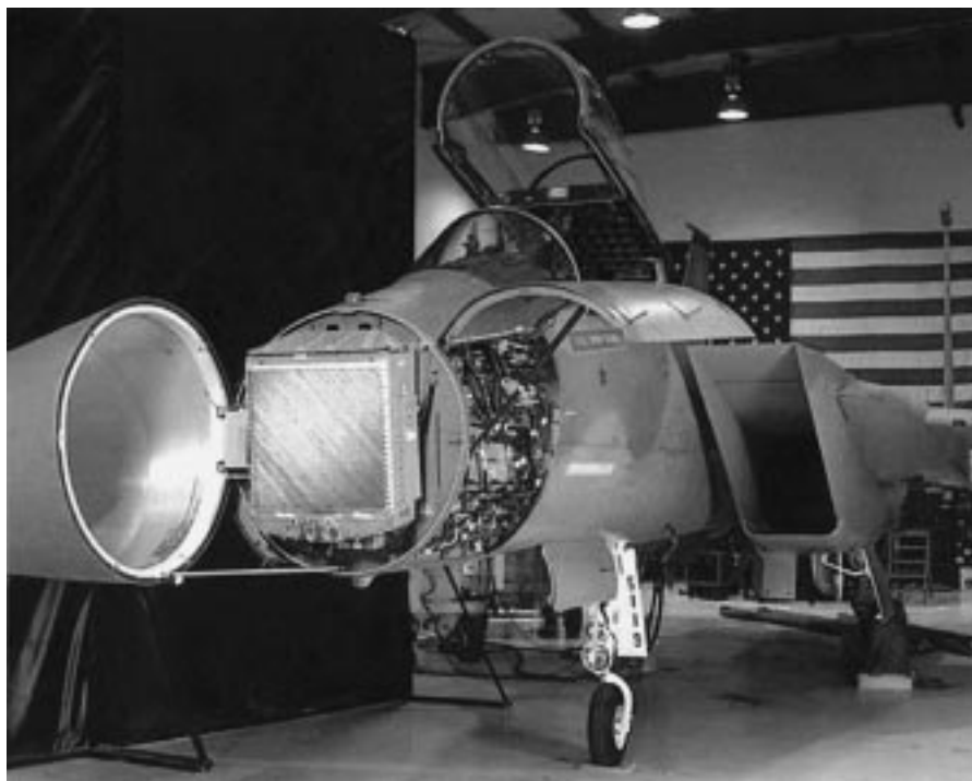
Fig. 14. 18 operational F-15Cs have been refitted with Raytheon's APG-63(v)2 AESA.
